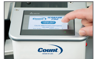
Touch Screen Controller
