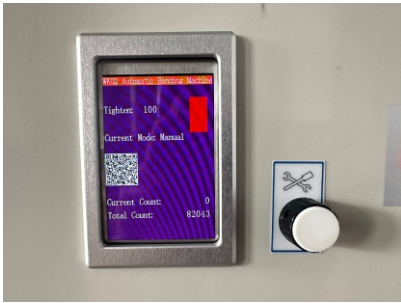
-Open HMI for Parameter Setting -Password Required Operation -With Counter
