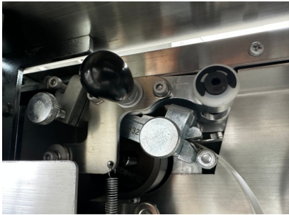
Loose 2 screws to Clear Jammed Band
